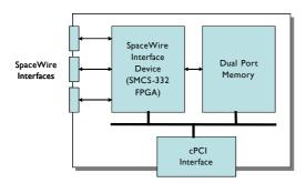
Figure 2: SpaceWire cPCI block diagram
