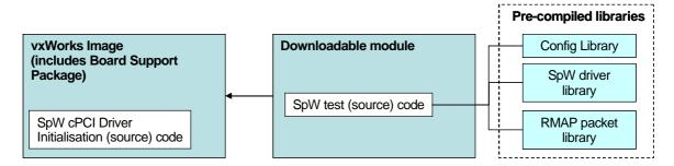
Figure 1: SpaceWire VxWorks driver software components
