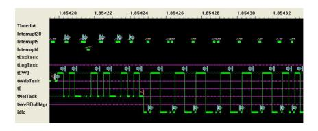
Figure 4: SpaceWire cPCI-2 driver task scheduling during a single loopback test with packet size of 100 bytes
