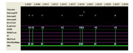
Figure 3: SpaceWire cPCI-2 driver task scheduling during a single loopback test with packet size of 20,000 bytes
