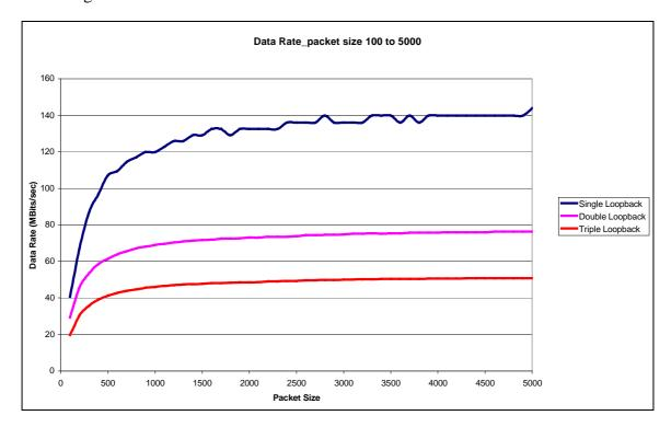
Figure 5: SpaceWire cPCI VxWorks data transfer rates with varying packet size
