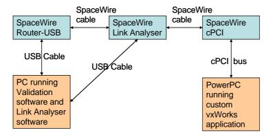
Figure 6: Jitter test setup diagram
