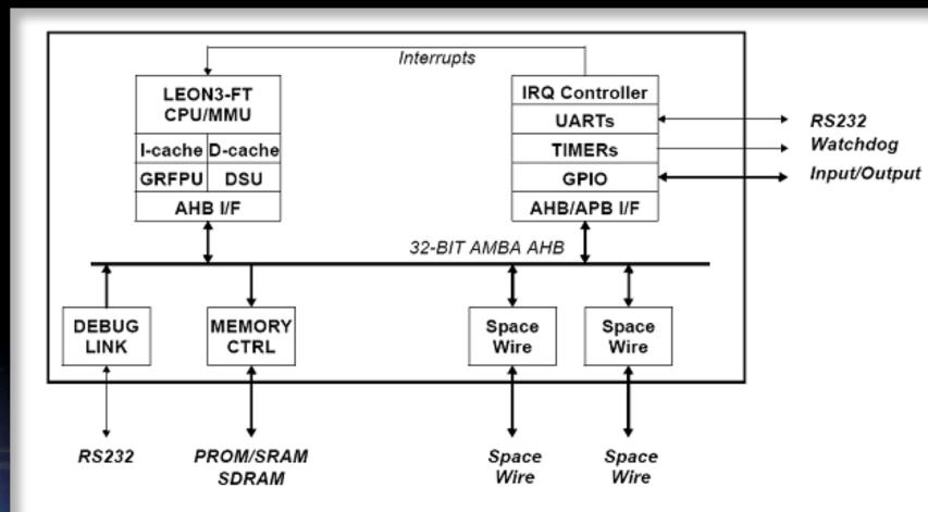
ESA activity with the aim to implement and characterize the complex ASIC on radiation-hard UMC 180 nm technology (DARE)
