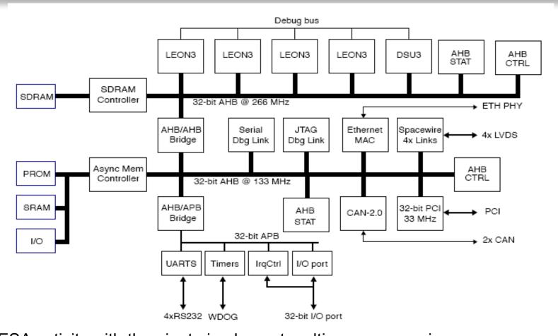
ESA activity with the aim to implement multi-core processing ST 90 nm technology as baseline
