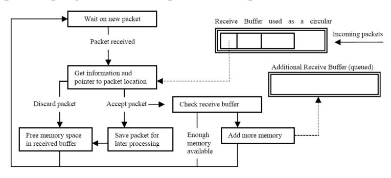
Note that it is possible to keep current packet in the Driver receive buffer and only free memory used by old packets.
