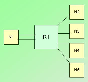
N1 – onboard computer system. It handles all distributed interrupts and it's the destination off all packets
